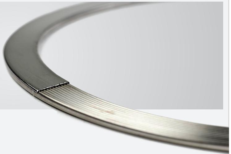
Manufactured from solid metal, CANFLEX® Cammprofile gaskets combine all of the desirable qualities of a solid metal gasket with the added advantages of a reduced area of contact, resulting in lower stress values required to achieve a seal. As a standard, flexible graphite is bonded to each face due to its superior sealing characteristics. Other metallurgies and soft gasket sealing materials are available in order to accommodate specific chemical and temperature service requirements.
