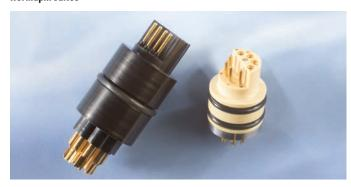
Hermaphrodite connectors have mating surfaces with both male and female contacts that are mated into identical opposite fittings for a keyed (fail-proof) installation. Our hermaphrodite connectors are rated to 204°C (399°F) and 20,000 psi. Multiple pin counts are available on request.
