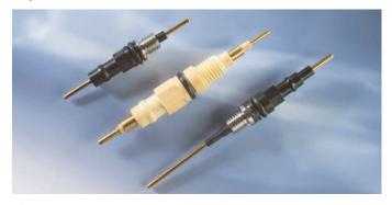
Single-pin and coaxial Seal-Connect® designs provide secure, reliable power and signal transmission in rugged environments. They are most commonly offered in Arlon® 2000 or 3000 XT materials, with copper alloy contacts, unless otherwise specified.
