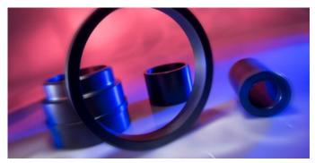
Greene, Tweed's WR<sup>®</sup> 300 is composed of PEEK reinforced with short, random carbon fibers with a temperature range from subzero to 275°F (135°C). WR<sup>®</sup> 300 is suitable for general wear resistance applications and is often used in pump bushings and cases or impeller wear rings.
