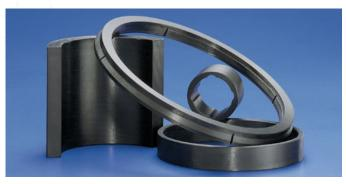
Greene, Tweed's WR<sup>®</sup> 525 is made of PEEK reinforced with continuous hoop-wound carbon fibers and is ideal for use as impeller wear rings, bushings, and case wear rings in high-pressure and high-temperature (HPHT) conditions. WR<sup>®</sup> 525's temperature range of subzero to 525°F (274°C) is suitable for stationary and rotating applications and allows users to increase efficiency with tighter wear ring clearances and decrease potential damage.
