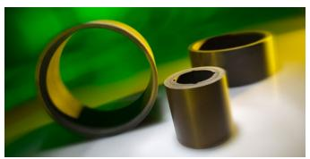
Greene, Tweed's AR<sup>®</sup> 1 is made of filled PTFE and is engineered to be abrasion-resistant. It can operate from subzero conditions up to 120°F (49°C), and is suitable for general abrasive resistance applications, particularly vertical pumps.
