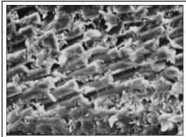
SEM photo of standard glass-reinforced epoxy magnified at 550 times
