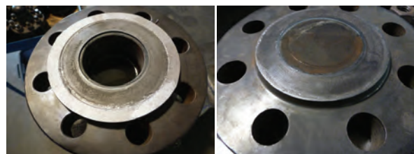
Figure 1: Gasket in 550°F steam treated with Thomson SURE-RELEASE® anti-stick treatment.
